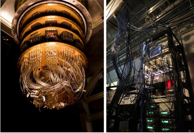
Fig. 2: A side by side view of a dilution refrigerator and electronic rack for Google’s quantum computer.
